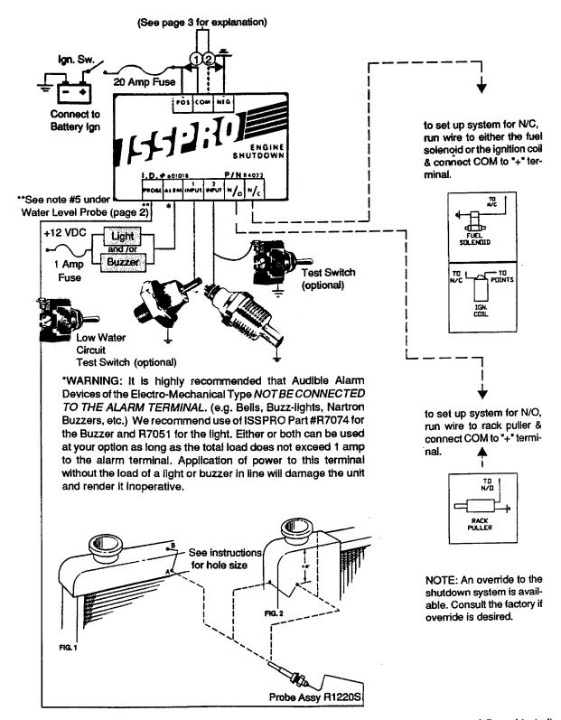
\*WARNING: Incorrect wiring can damage the shutdown box. Read ALL directions carefully and test after installation to insure proper function and to keep your limited warranty in effect!
